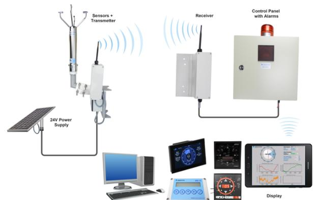
Figure 4: High wind-alarm solutions, advanced options for port operations, technology includes communication, multi-level alarms, data-logging, and power configuration (Source: Wind-Alarms website).
