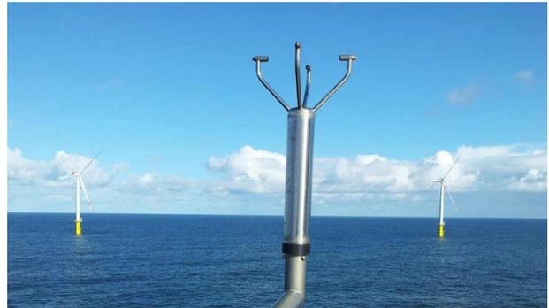
Figure 2: Gill Instruments Wind Observer II, wind speed sensor ideal for use in extreme environments, high accuracy sensor for low maintenance maritime applications (Source: Gill-Instruments website).
